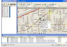
Along that same line, the GPS System could provide more safety in “man-down” situations. A service worker could wear an “alert fob” on a necklace while working, and if he becomes injured and is within 300 feet of his vehicle, pressing the alert button could have the vehicle's GPS Unit call several people for help. Those receiving such calls would see the vehicle ID and its current GPS position on their cell phone.
