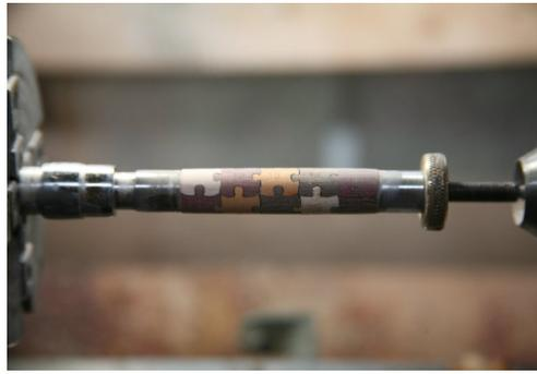
Place the barrel with bushings on the mandrel and place in lathe. Use 180 grit sandpaper to sand the barrel to the desired shape. While sanding place a couple of ( thin ) CA glue drops on the barrel, that would fill all the small gaps in between the puzzle pieces and ensure a great finish product. Use progressively finer sandpaper until you are satisfied with the finish.
