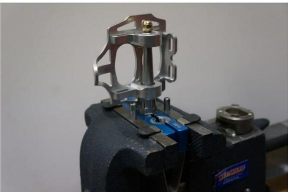
Fig.17 Pedal axle vice with pedal.
