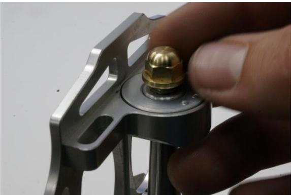
Fig.16 Thread on acorn nut.
