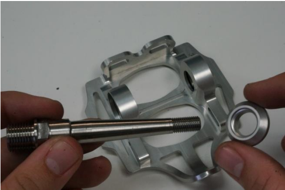
Fig.10 Installing dust shield .
