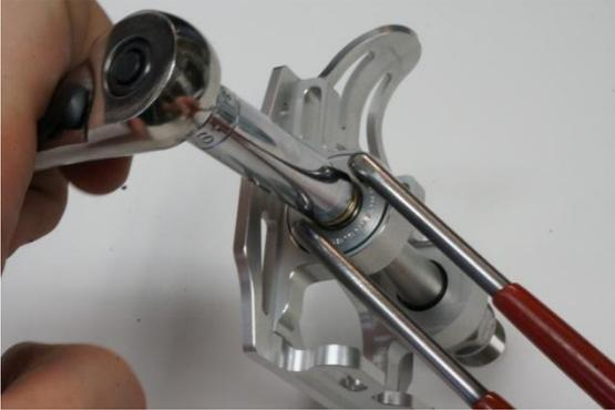
Fig.1 Loosening acorn nut.
