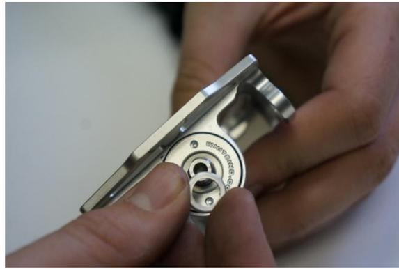
Fig.15 Slip on small washer.
