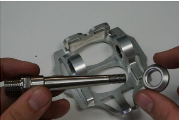
Fig.10 Installing dust shield .
