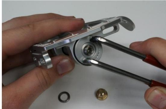
Fig.2 Removing adjustable locking collar.
