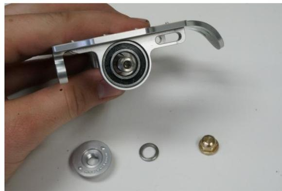
Fig.13 Spindle installed.
