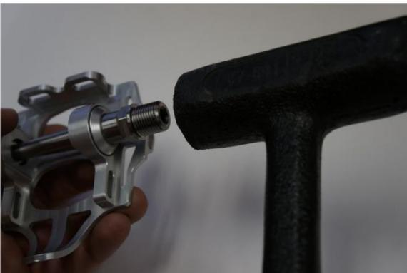
Fig.20 Adjustment with mallet.
