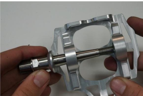
Fig.12 Inserting spindle into platform
