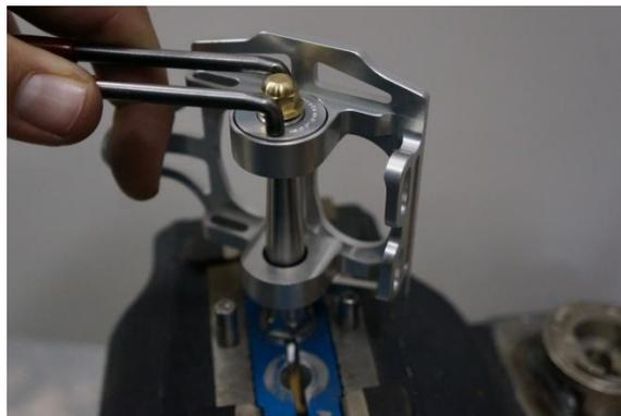
Fig.18 Snug down adjustable locking collar .
