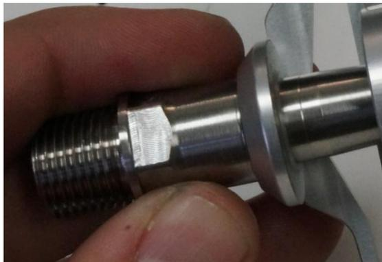
Fig.11 Proper orientation for dust shield.
