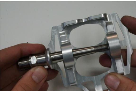
Fig.3 Slide out spindle.
