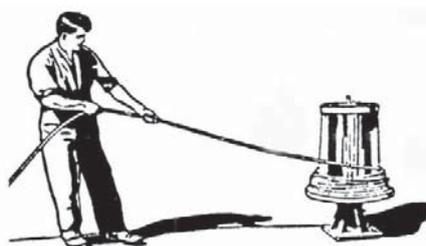
**Coils** - Place the coil over a turntable, release the ties and pull the free end as above. Alternatively, the coil may be rolled along the ground, leaving the rope lying straight on the ground, although manhandling a long length of wire rope in a coil can be very difficult.
