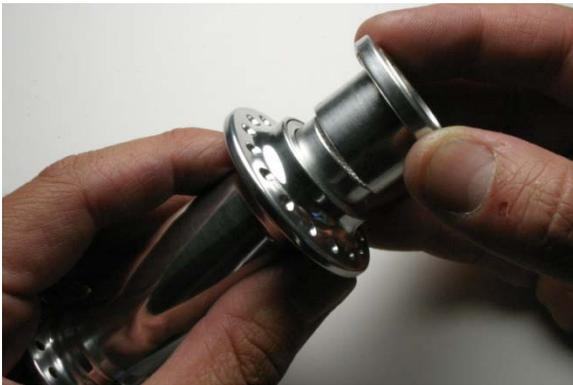
Fig.14 Slip tubing/socket over axle end.
