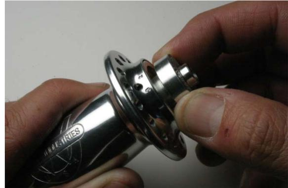
Fig.2 Removing adjustable axle end.
