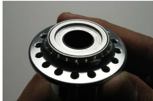
Fig.11 Proper orientation for collar.
