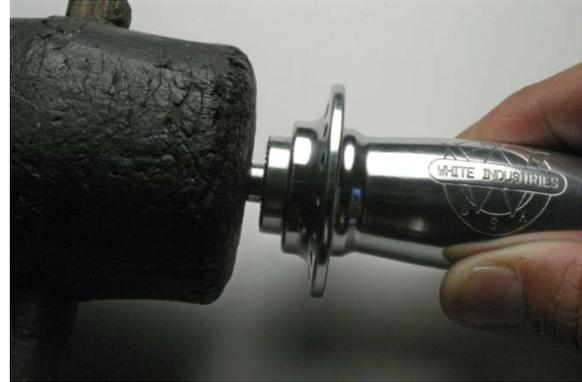
Fig.9 Tap axle end to fully seat.
