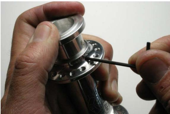
Fig.16 Tighten set screws.
