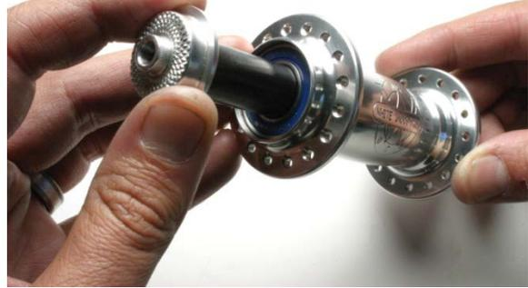
Fig.5 Removing axle from hub shell.
