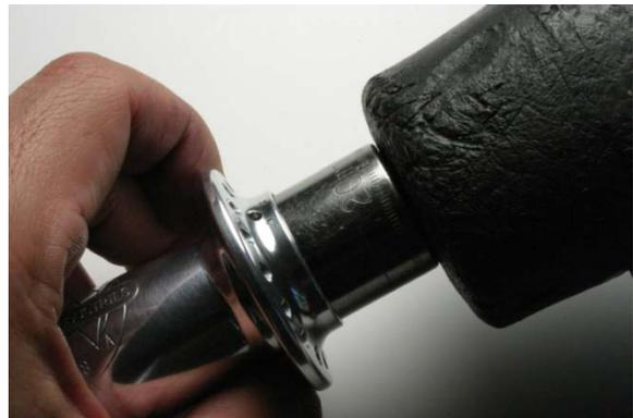
Fig.7 Fully seat bearing in bore.
