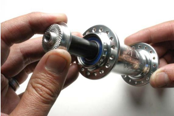
Fig.8 Installing axle with pressed on end.
