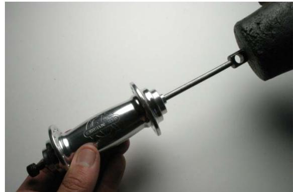
Fig.4 Tapping skewer to remove axle end.
