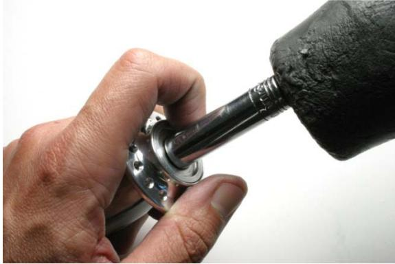
Fig.4 Tapping axle through hub shell.
