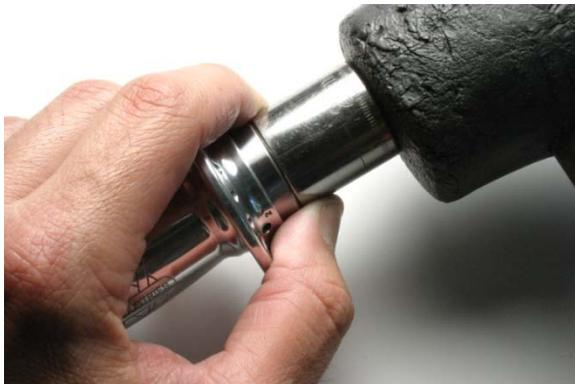
Fig.6 Tapping bearing into bore.
