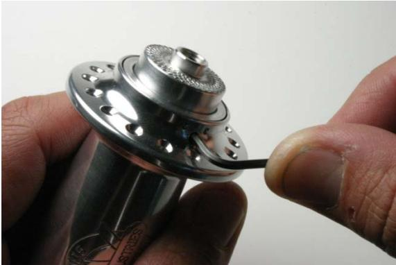
Fig.1 Loosening set screws.
