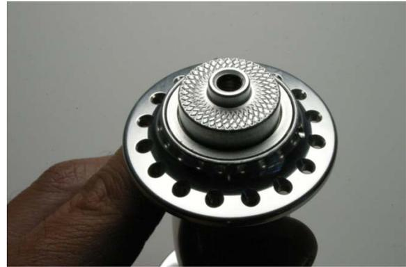
Fig.13 Axle end installed.
