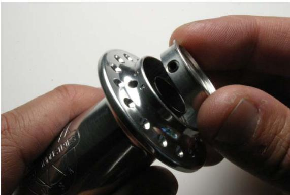
Fig.10 Installing adjusting collar.
