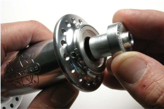
Fig.12 Inserting axle end.
