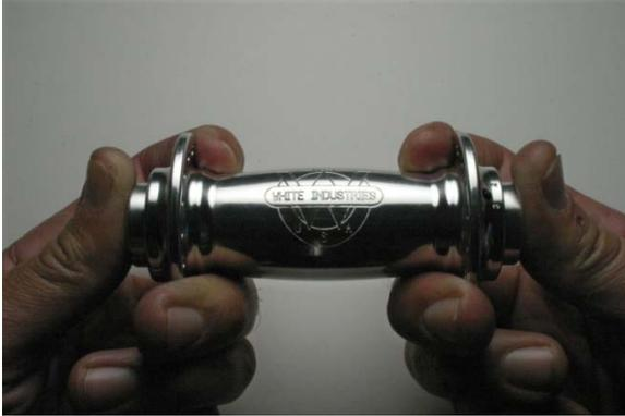
Fig.17 Checking for play in hub.
