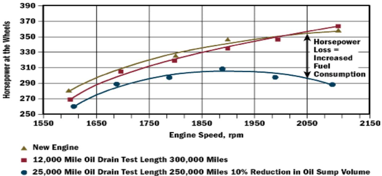
● **25,000 Mile Oil Drain Test Length 250,000 Miles 10% Reduction in Oil Sump Volume**
