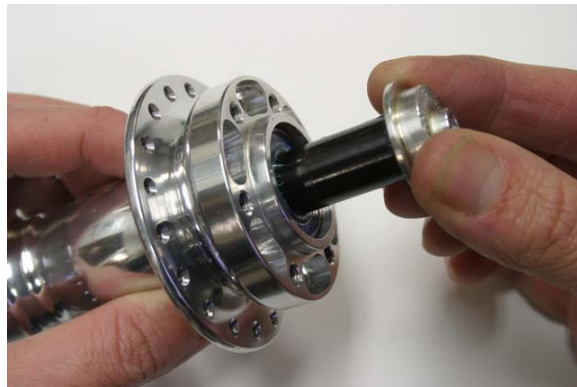
Fig.5 Removing axle from hub shell.
