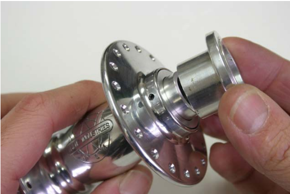
Fig.13 Slip tubing/socket over axle end.
