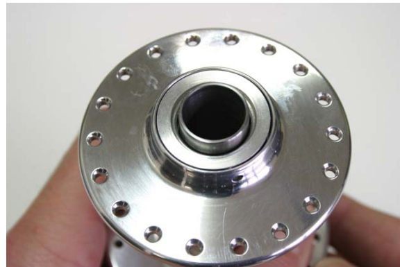
Fig.10 Proper orientation for collar.
