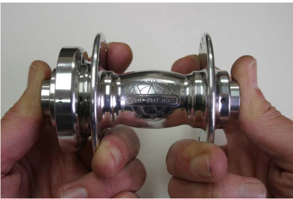
Fig.16 Checking for play in hub.
