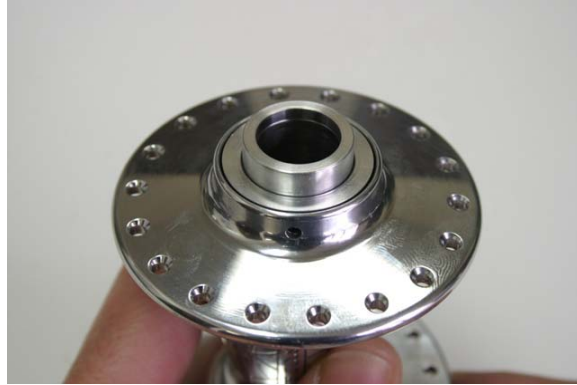
Fig.12 Axle end installed.
