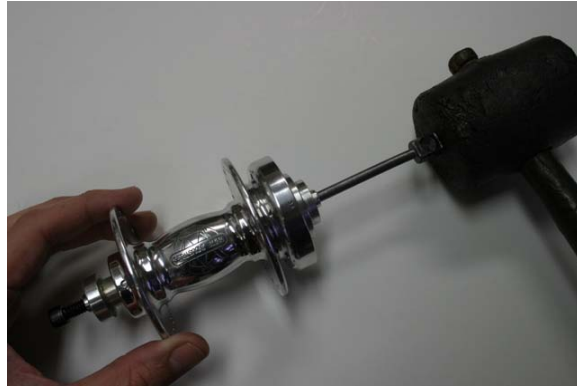
Fig.4 Tapping skewer to remove axle end.
