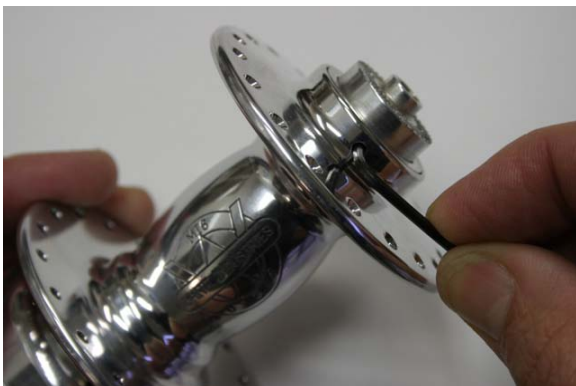
Fig.1 Loosening set screws.
