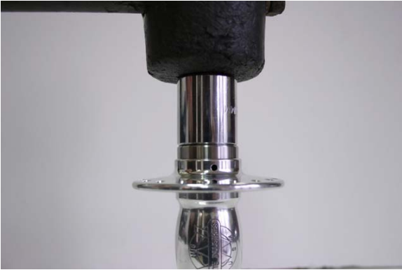
Fig.6 Tapping bearing into bore.
