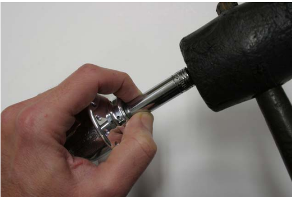
Fig.4 Tapping axle through hub shell.
