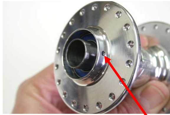
Fig.8 Axle visible on side with access hole.
