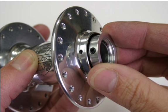
Fig.9 Installing adjusting collar.
