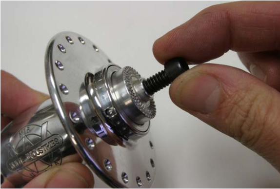
Fig.3 Threading in 6mm bolt.
