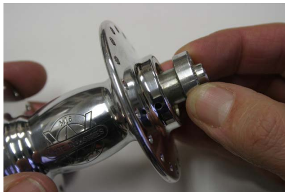
Fig.2 Removing adjustable axle end.
