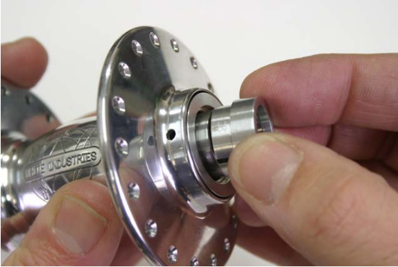
Fig.11 Inserting axle end.
