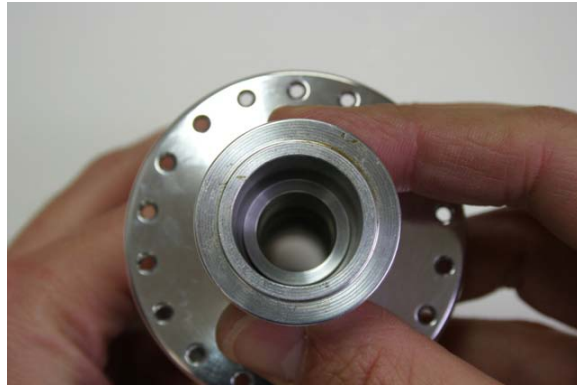
Fig.14 Tubing/socket resting on collar only.
