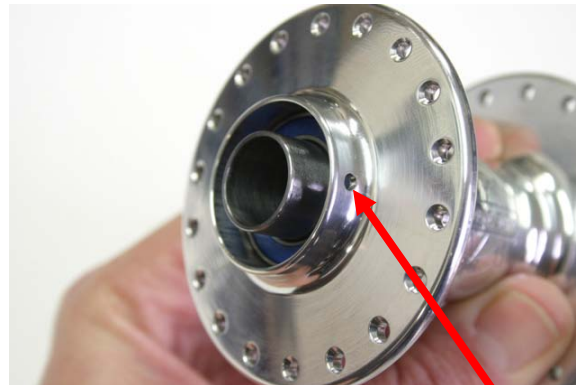
Fig.8 Axle visible on side with access hole.
