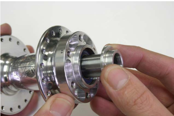
Fig.7 Installing axle with pressed on end.
