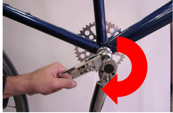
Fig.14. Tighten clockwise to 30 ft./lbs.
