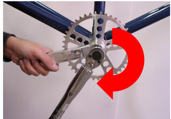
Fig.12 Tighten clockwise to 30 ft./lbs.
