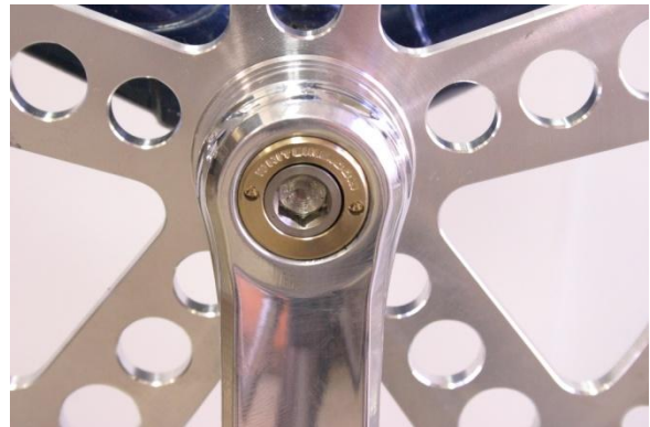
Fig.16 Bronze self-extracting ring installed.
