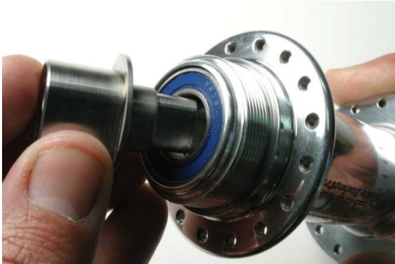
Fig.28 Install axle end into axle.
