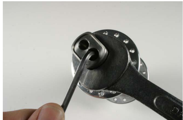
Fig.2 Removing 4mm bolt from axle end
