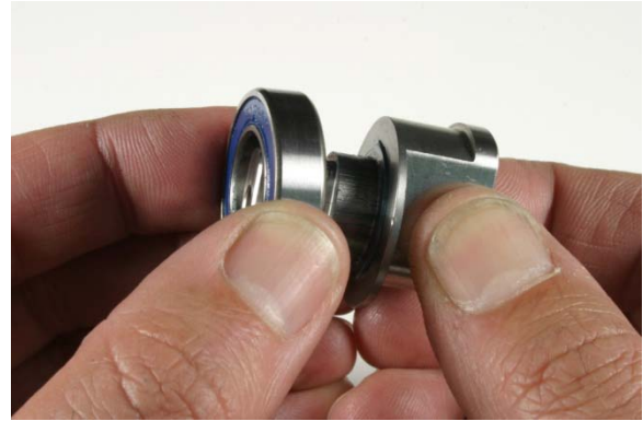
Fig.10 Removing bearing from axle end.
