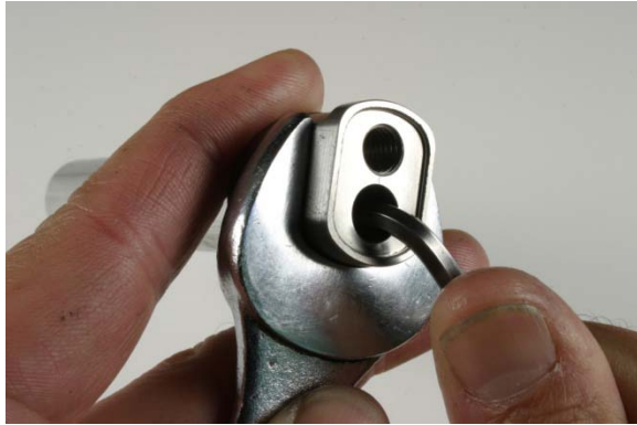
Fig.9 Removing 4mm bolt from axle end.
