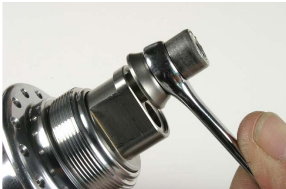
Fig.3 9mm wrench installed on axle end.
