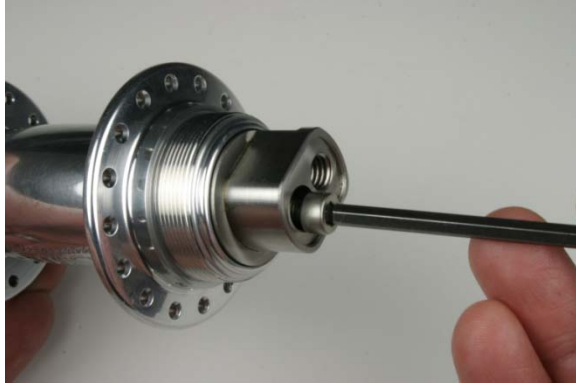
Fig.13 Installing 4mm bolt.
