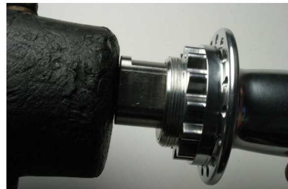
Fig.27 Tapping axle end to seat bearing.
