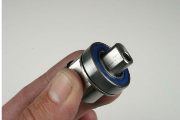
Fig.22 Installing new bearing.
