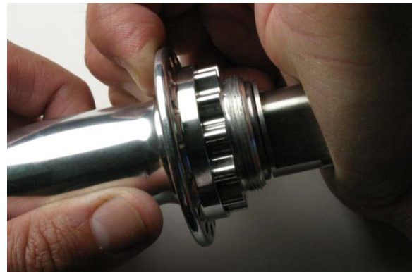
Fig.21 Tapping axle assembly into shell.
