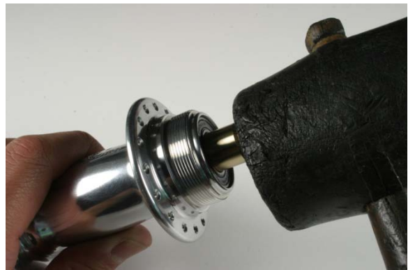
Fig.6 Driving out axle assembly.
