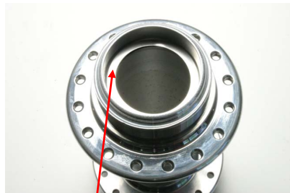
Fig.17 Washers on machined shoulder.
