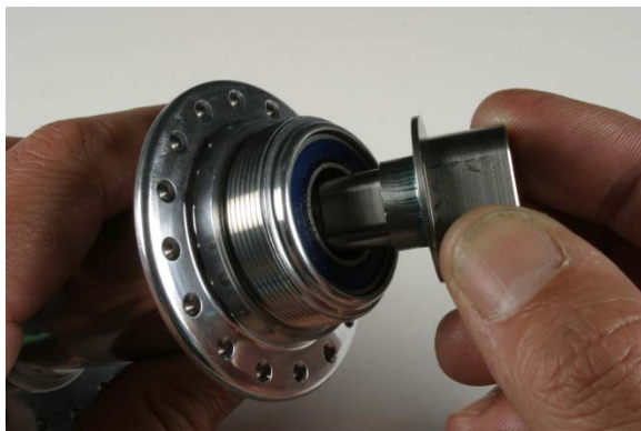
Fig.11 Inserting axle end.
