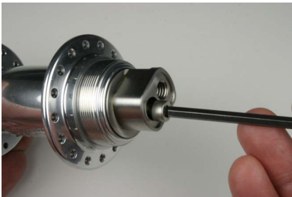
Fig.29 Tighten 4mm bolt.
