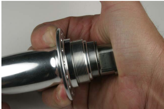
Fig.24 Pushing in axle assembly.
