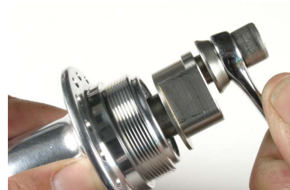
Fig.4 Removing axle end from hub.
