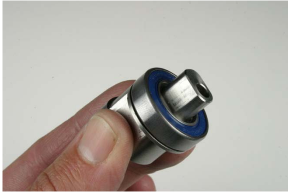
Fig.18 Installing new bearing.
