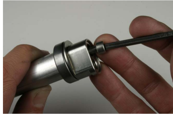
Fig.19 Installing 4mm bolt.
