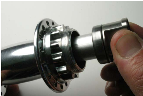
Fig.20 Inserting axle assembly.
