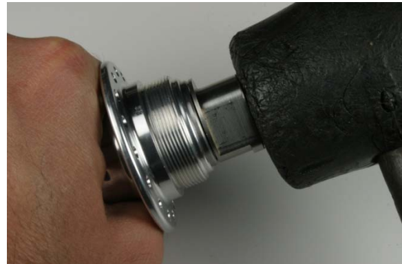
Fig.25 Tapping axle assembly into shell.
