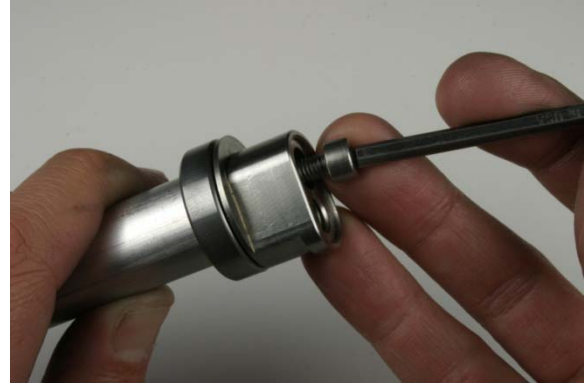
Fig.23 Installing 4mm bolt.
