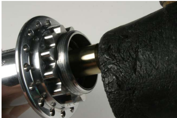
Fig.15 Driving out second bearing.
