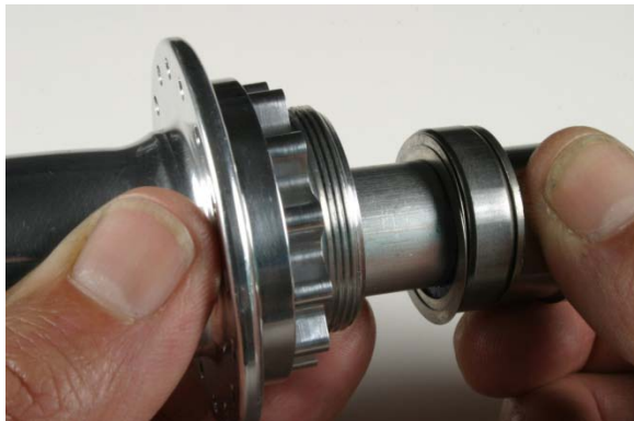
Fig.7 Withdrawing axle assembly.
