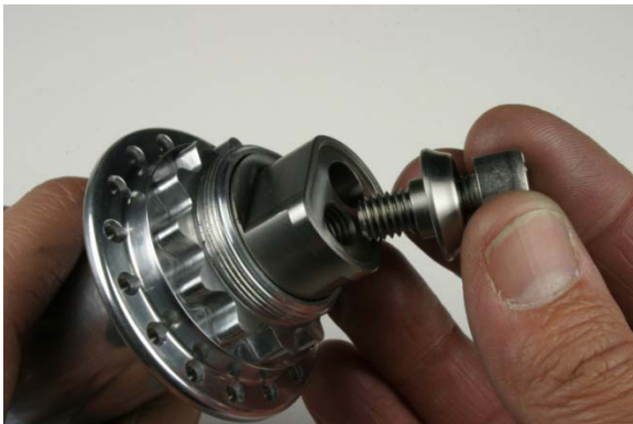
Fig.31 Installing axle bolt and washer.
