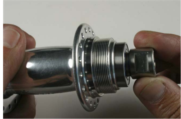
Fig.19 Finger tighten axle end.
