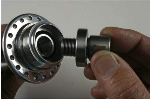
Fig.18 Installing axle end and bearing.
