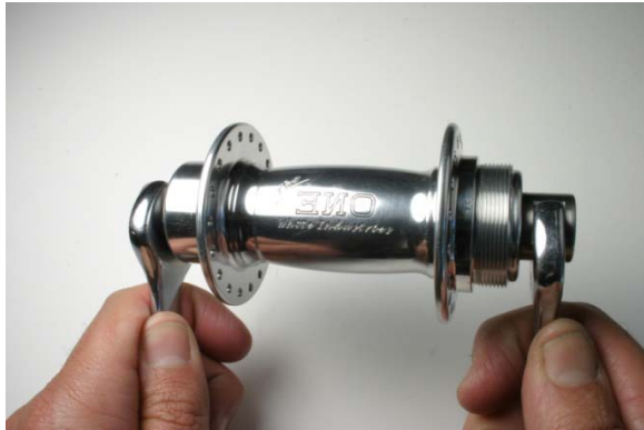
Fig.1 Loosening axle end.
