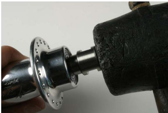
Fig.3 Tapping bearing out with mallet.
