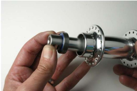
Fig.11 Removing axle/bearing assembly.
