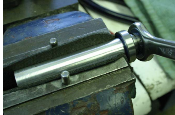
Fig.6 Axle in vise to remove axle end.
