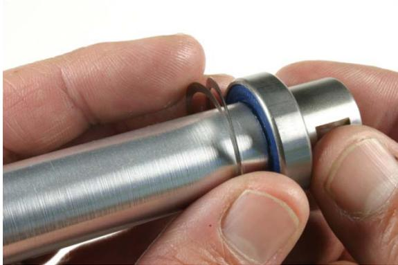
Fig.5 Washers between bearing and hub shell.
