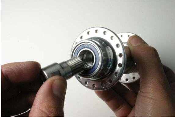
Fig.9 Installing axle end to capture bearing.
