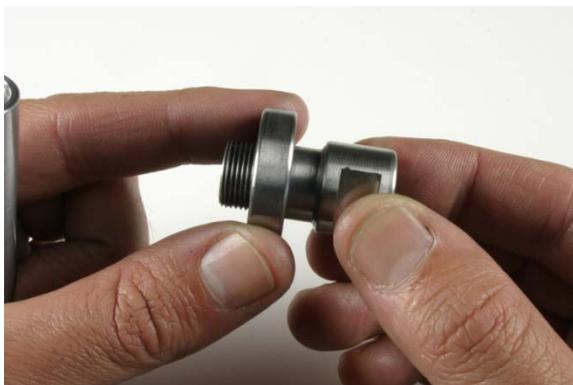
Fig.12 Placing bearing on axle end.
