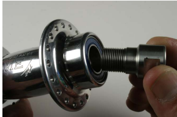
Fig.2 Removing axle end.
