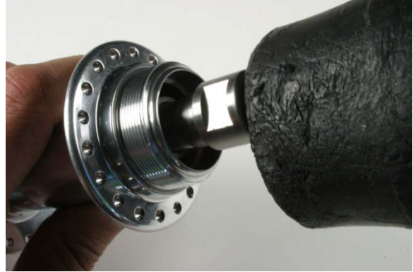
Fig.10 Driving out bearing with mallet.
