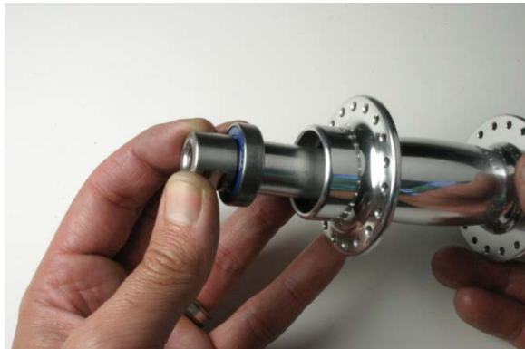
Fig.11 Removing axle/bearing assembly.
