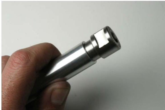
Fig.7 Axle end installed on axle.
