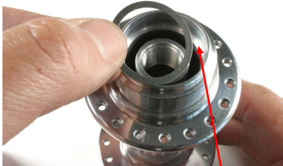
Fig.16 Placing thin washers on shoulder.
