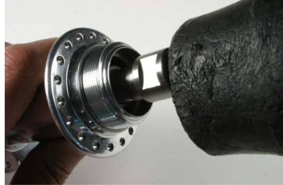
Fig.10 Driving out bearing with mallet.
