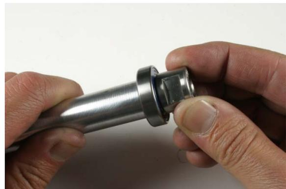
Fig.13 Threading axle end into axle.
