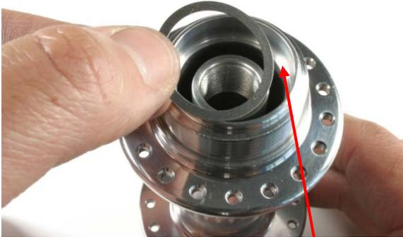
Fig.16 Placing thin washers on shoulder.
