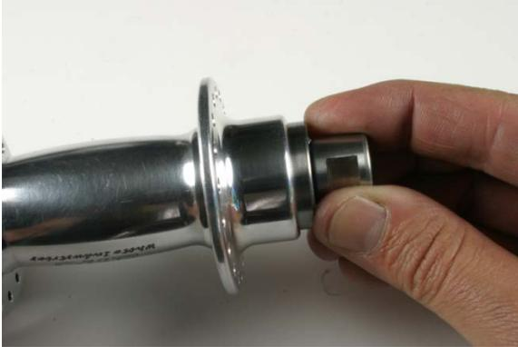
Fig.14 Starting bearing into bore.
