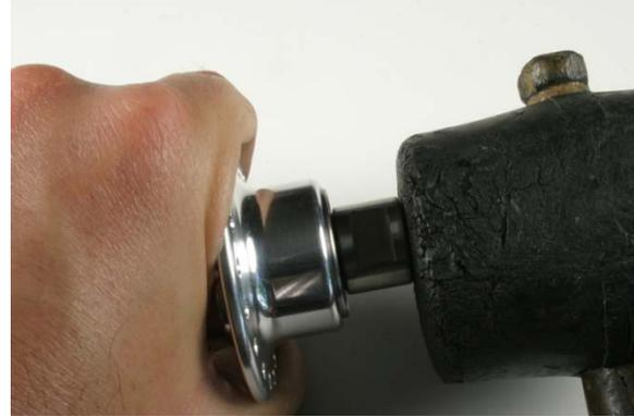
Fig.15 Tapping bearing into bore.
