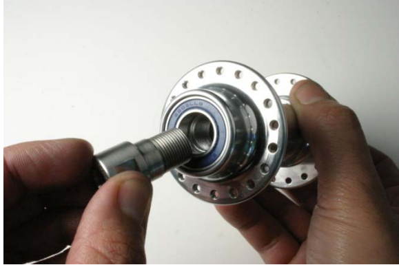
Fig.9 Installing axle end to capture bearing.
