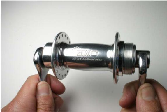
Fig.1 Loosening axle end.
