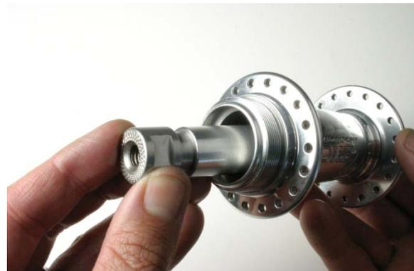
Fig.8 Axle going into hub shell.
