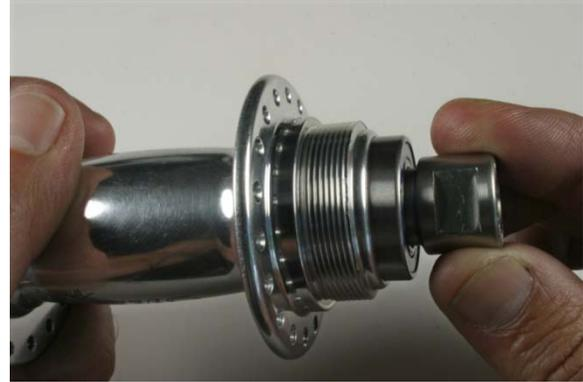
Fig.19 Finger tighten axle end.
