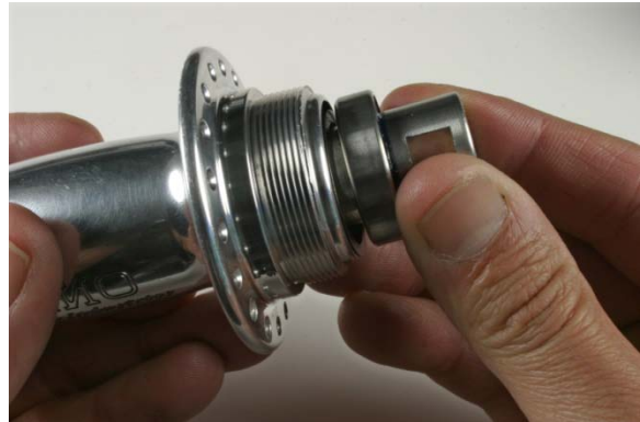
Fig.4 Withdrawing axle/bearing assembly.
