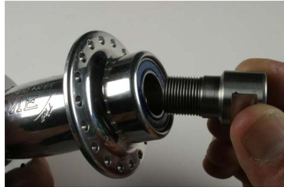
Fig.2 Removing axle end.
