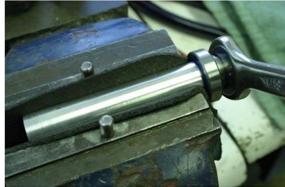
Fig.6 Axle in vise to remove axle end.
