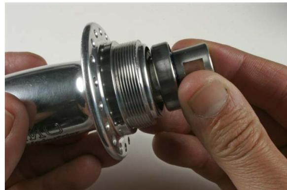
Fig.4 Withdrawing axle/bearing assembly.
