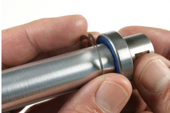
Fig.5 Washers between bearing and hub shell.
