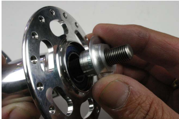
Fig.14 Installing aluminum cone nut.
