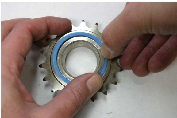
Fig. 22 Push rear seal into place.
