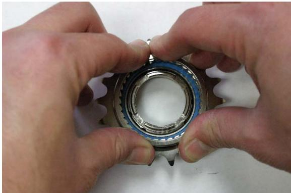
Fig. 14 Seat bearing fully into bore.
