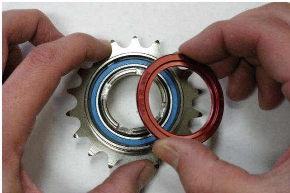
Fig. 20 Install lock ring.
