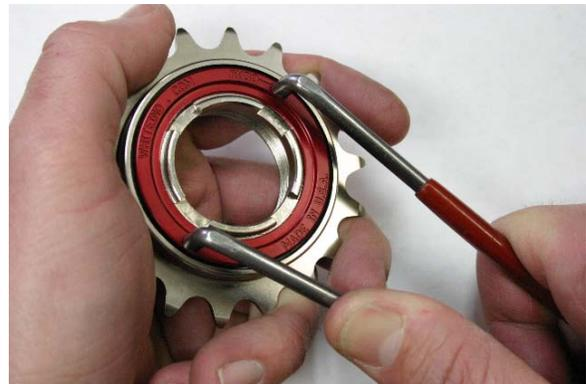
Fig. 21 Tighten lock ring to left.
