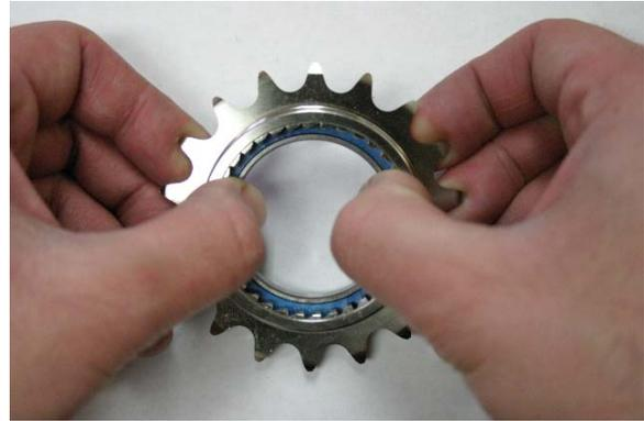
Fig. 9 Pressing out bearing.
