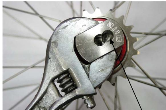
Fig. 2 Thread ENO axle bolt into here.
