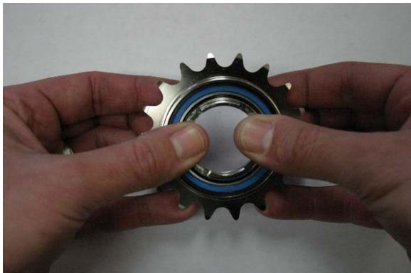
Fig. 5 Pressing out inner driver
