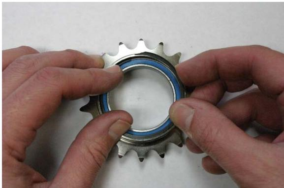
Fig. 16 Install snap ring.
