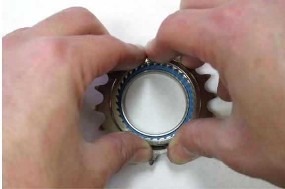
Fig. 12 Pressing bearing into bore.
