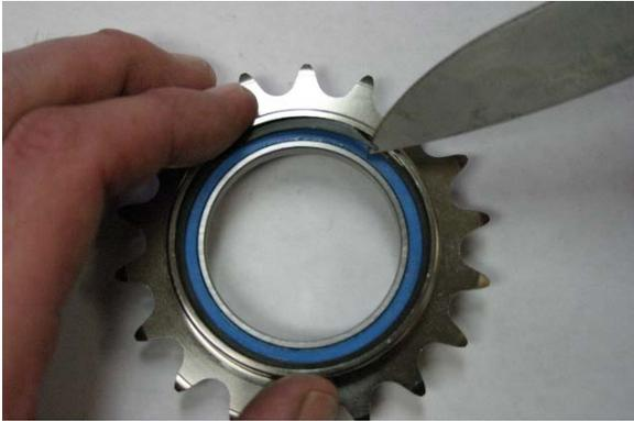
Fig. 8 Removing snap ring.
