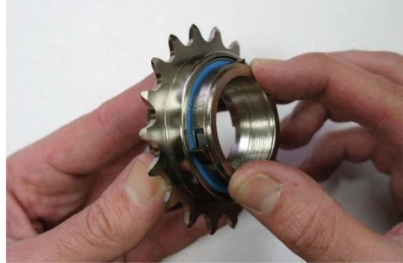
Fig. 13 Place inner driver into bearing.
