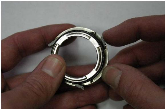
Fig. 7 Checking pawls of inner driver
