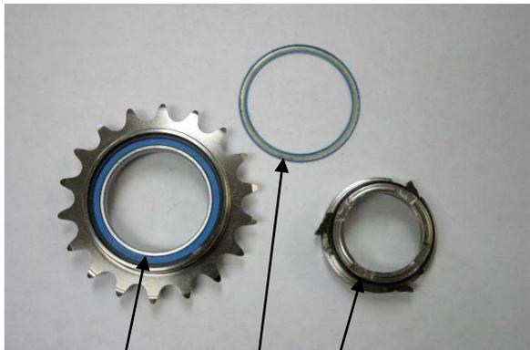
Fig. 6 Bearing, rear seal, inner driver
