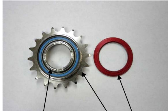
Fig. 4 Inner driver, outer gear, lock ring
