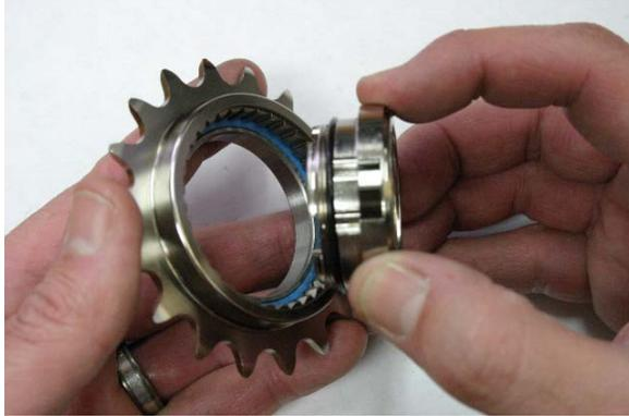
Fig. 18 Insert inner driver into outer gear.
