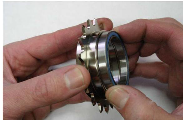
Fig. 11 Start bearing into bore.
