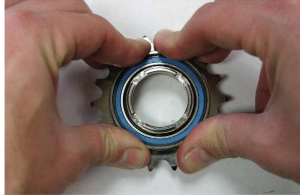
Fig. 19 Press down to seat inner driver.
