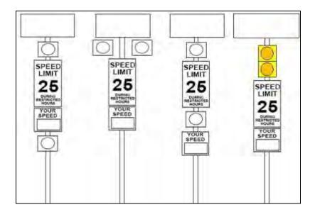
The box at the top is a solar panel powering the device. Installing these devices in clear view for motorists is part of a "gateway" treatment as motorists enter West 70<sup>th</sup> Street from all directions. The flashing lights can be timed to operate all day or only during school hours.
