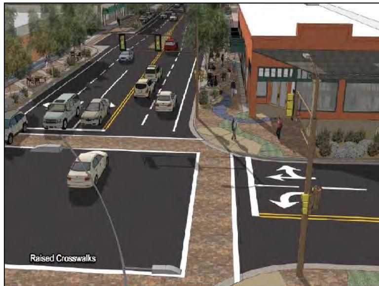
**Proven to:** Reduce crashes of turning and through vehicles at signalized intersections.<sup>17</sup>
