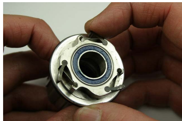
Fig.10 Checking pawl movement.
