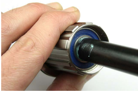
Fig.15 Insert axle into freehub body.
