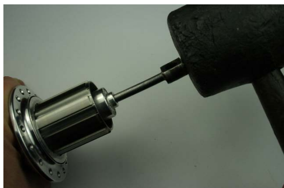
Fig.4 Tapping QR to free axle end.
