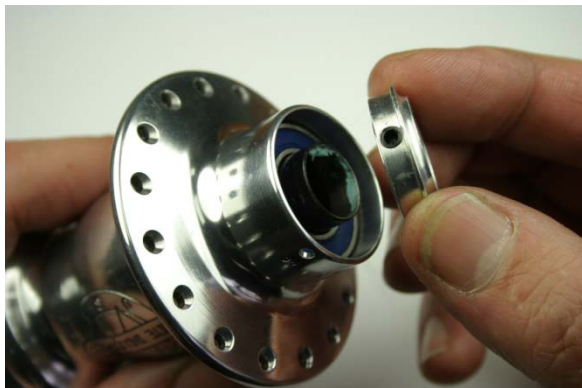
Fig.21 Installing adjusting collar.
