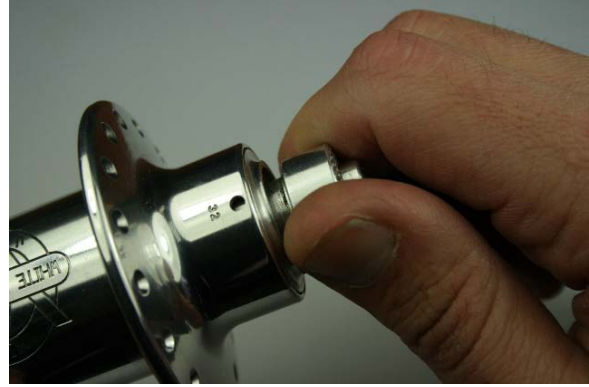
Fig.2 Remove axle end.
