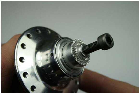
Fig.3 Thread 6mm bolt into axle end.
