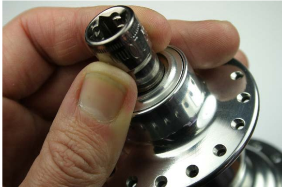
Fig.5 Place socket or dowel against axle.
