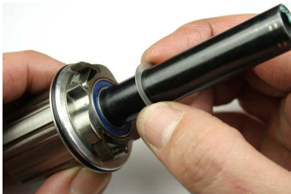
Fig.17 Install thrust washer.
