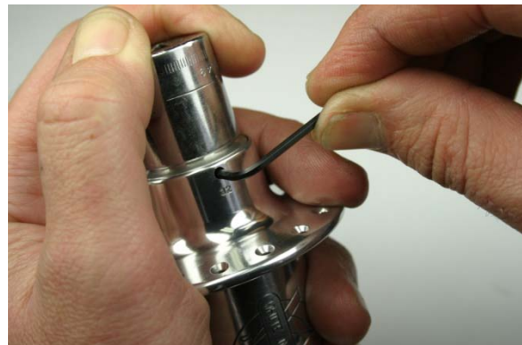
Fig.24 Press collar while tightening set screws.
