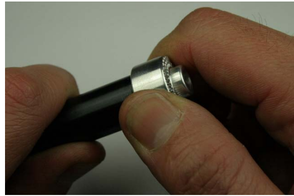
Fig.14 Checking fit of pressed on axle end.
