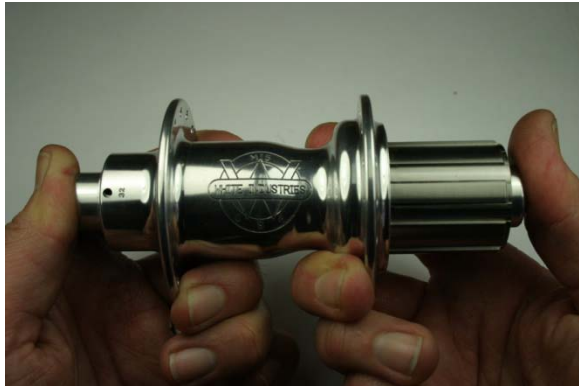
Fig.25 Checking hub for play.
