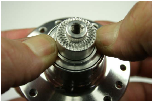
Fig.23 Press down on adjusting collar.
