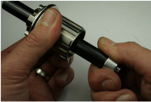
Fig.13 Pull axle out of freehub body.
