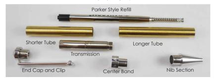
Layout your blank so that the longer tube section is at the nib end and cut blank to size. Both sections will use the same 8mm drill bit (or 5/16"). Once you have drilled your holes, glued your tubes in and squared off the ends, turn the blanks down even with the bushings. There are no tennons or special cuts needed. Once you have turned and finished both sections of your pen, proceed to the assembly instructions below.
